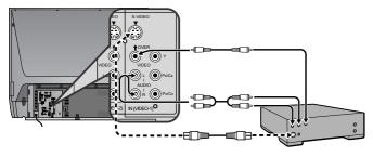
Note that the connection with a video cable will be ignored in case you connect a VCR to the TV with both video cable and S-VIDEO cable.
